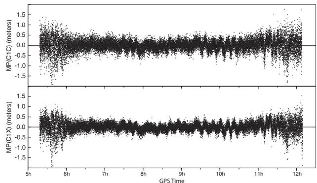
**FIGURE 4** Multipath linear combination (L1 pseudorange and L1 and L2 carrier phase) of the SVN74 L1 C/A-code (top) and L1C signal (bottom) from 1-Hz data of February 3, 2019, tracked with a Javad TRE-G3TH receiver at the Geodetic Observatory Wettzell.
